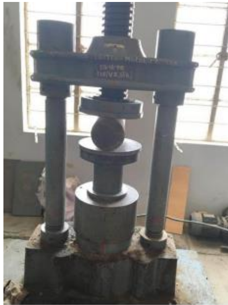
Split tensile strength of cylinder under test
