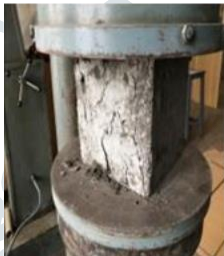
Compressive Strength Test
