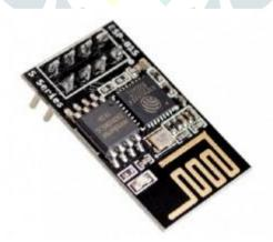
**Wireless communication modules**: These modules provide connectivity between the sensors and the cloudbased data analytics platforms, allowing for real-time monitoring and analysis of water quality and usage.
