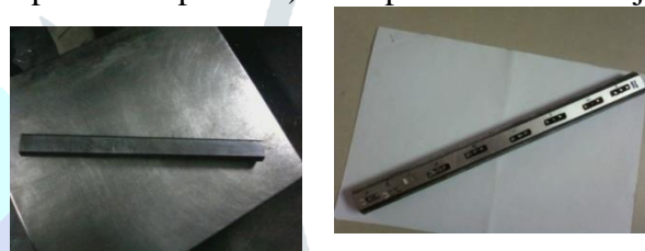
Fig.2.1 H-13 Work piece before and after machining with tool
