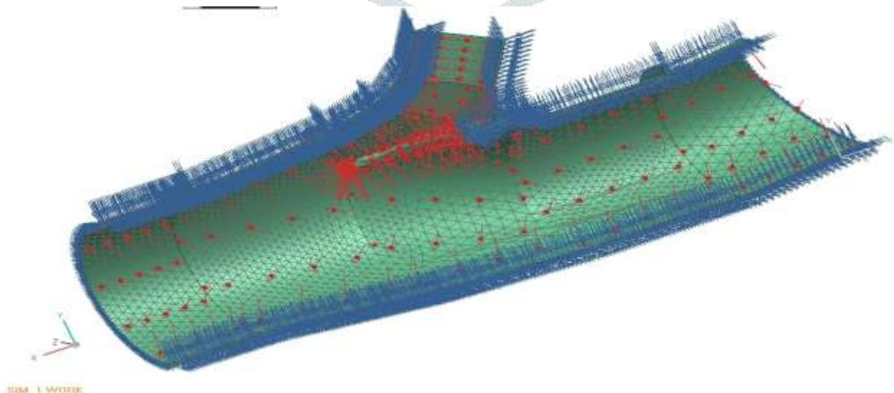
Figure 3.4.1 Loading & Boundary condition on Wye-1
