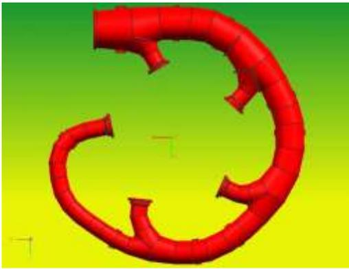
Figure 5.1.1 Solid Model of Distributor
