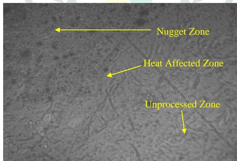
Figure 3 Optical micrograph of surface of the fabricated composite.
