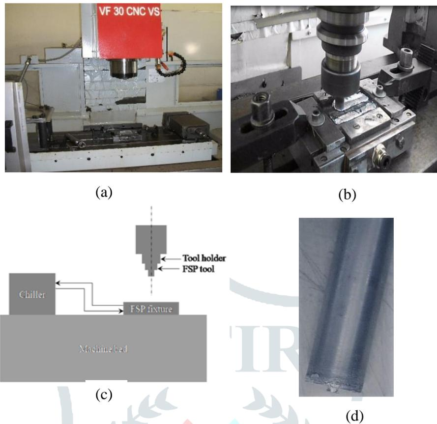
Figure 1 (a) Actual set-up on CNC vertical milling machine (b) FSP operation (c) Line diagram of the set-up used and (d) FSP tool used in experimentation.
