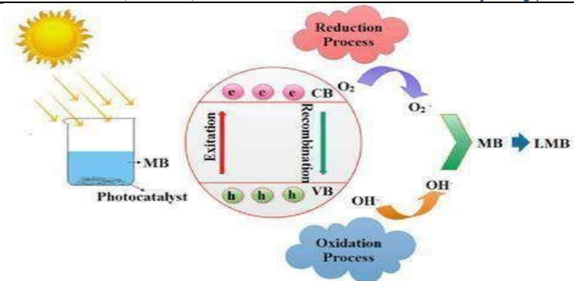
Fig. 2: Schematic representation of photo catalytic activity process
