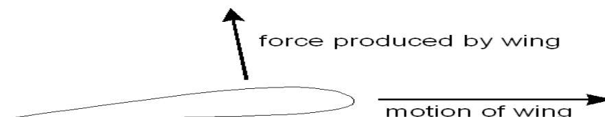
Fig.3.3.1. Airplane wing in forward flight produces lift
