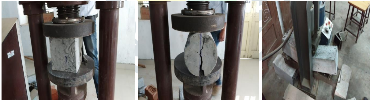
Fig. 3, 4, 5: Compressive Strength test, Split Tensile test, Flexural Strength test
