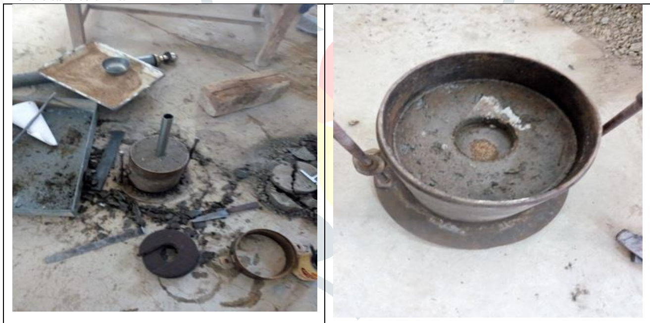
Fig.1 CBR test with sand column
