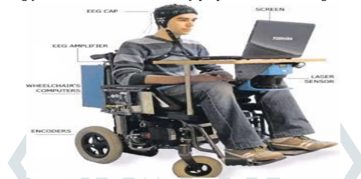
fig 4: mind controlled wheelchair
