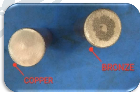
fig.7- Machining Surface of Electrodes after machining
