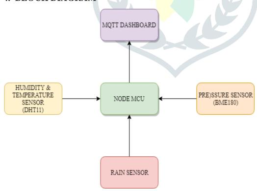
Figure 1: Block diagram of IoT and Arduino Based Weather Station.
