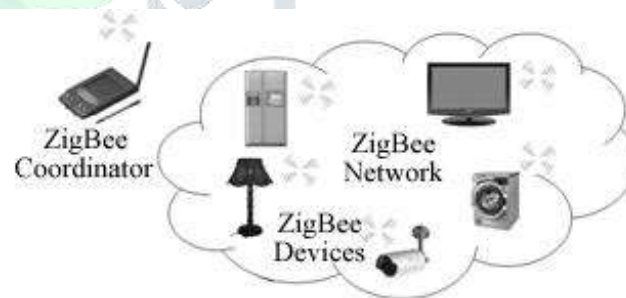
Fig. 2. Zigbee Home Automation Architecture.
