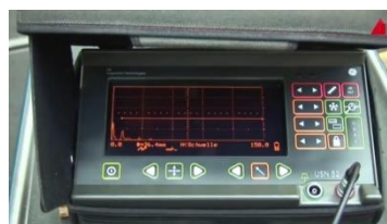
Fig 7.7: Ultrasonic testing flaw indication showing less flaws
