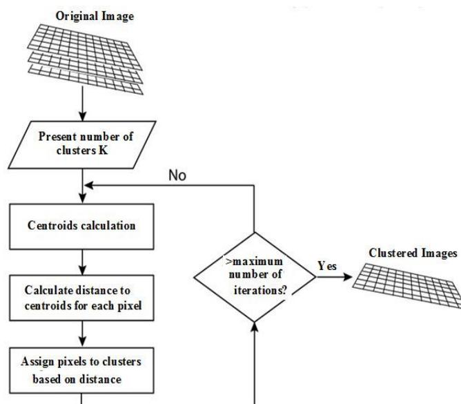
Fig. 3. K-means Clustering Algorithm.
