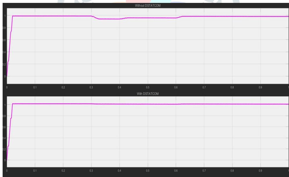
Figure 8: Line to Ground fault condition with and without D-STATCOM
