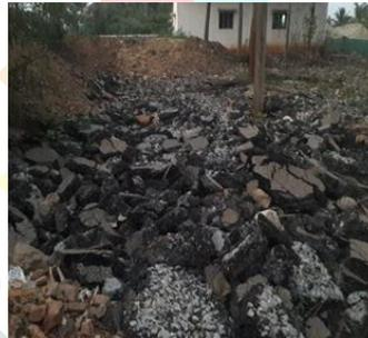
**Fig 5.2:** Reclaimed Asphalt Pavement**Table 5.2:** Test Results on RAP
