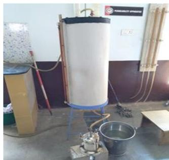
Fig 5.1: Constant Head Permeability Apparatus
