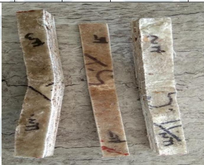
**Fig11-After Flexural Test Specimen**
