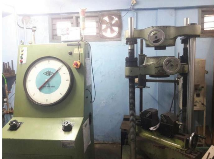
**Fig.7- Universal Testing Machine**
