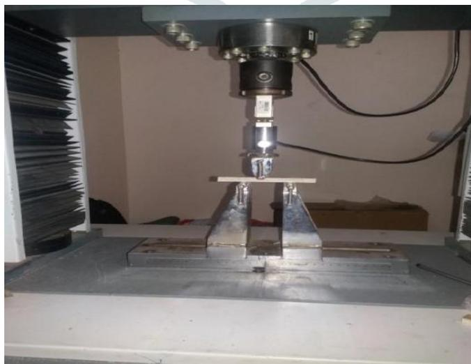
**Fig.8- Flexural Testing Machine**
