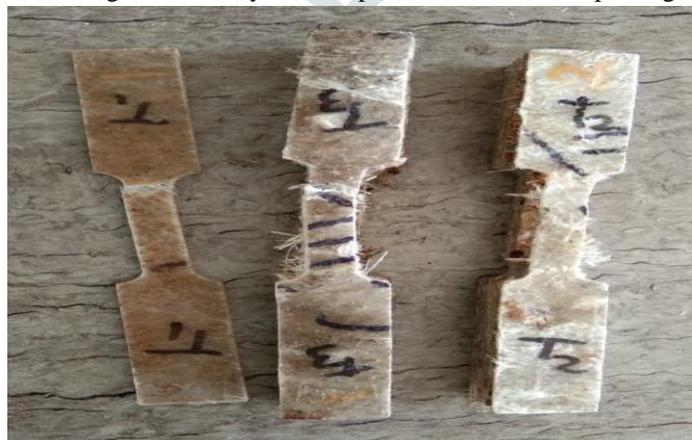
Fig10-After Tensile Test Specimen
