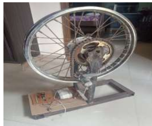
Fig 8: out put voltage of Regenerative Braking System up to 11.7v
