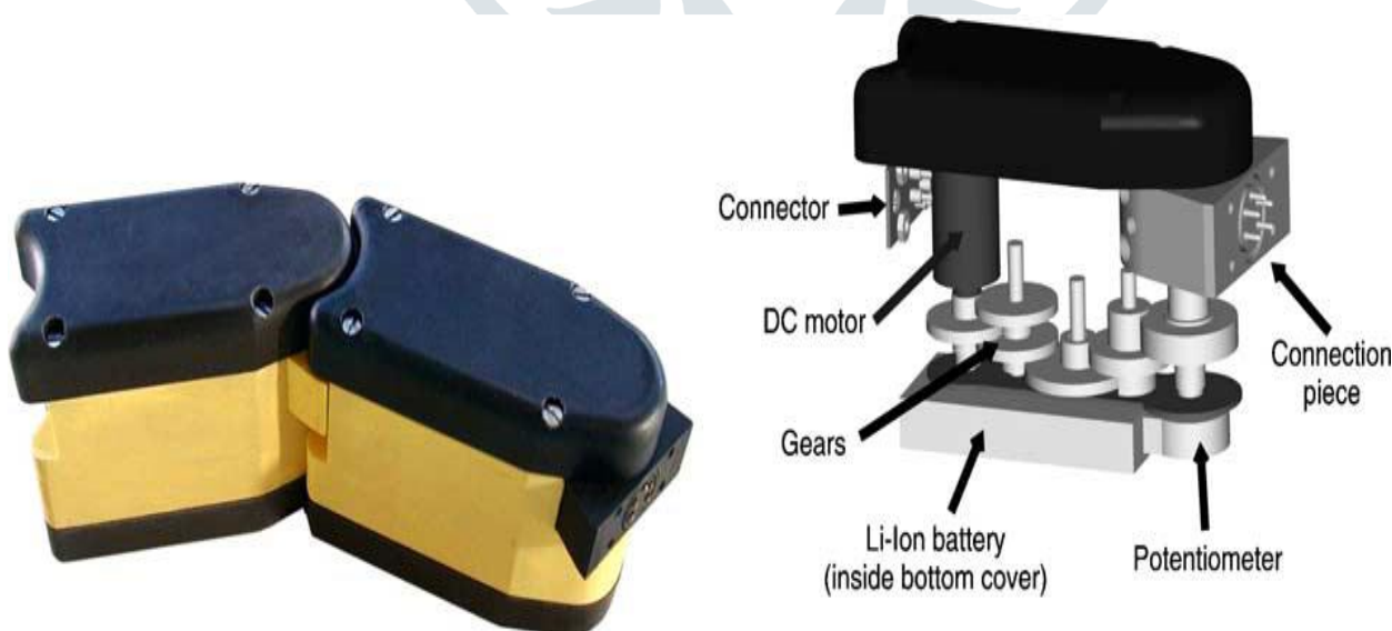
Fig.15: Design of single link of AmphiBot [2]
