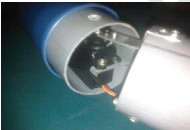
Fig.7: Link mechanism of SNAKEY [8]
