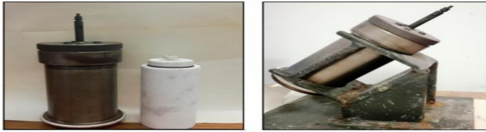
Fig Basic equipment for static sag test: (a) vertical setup aging cell and (b) 45° setup aging cell.
