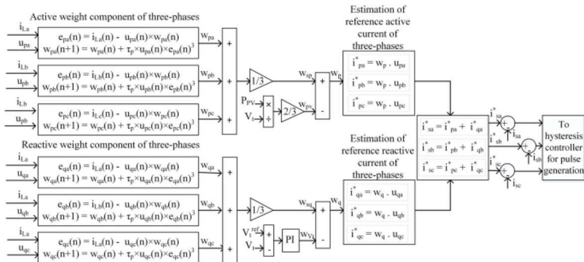
Fig. 2 Adaptive filter for power quality improvement
