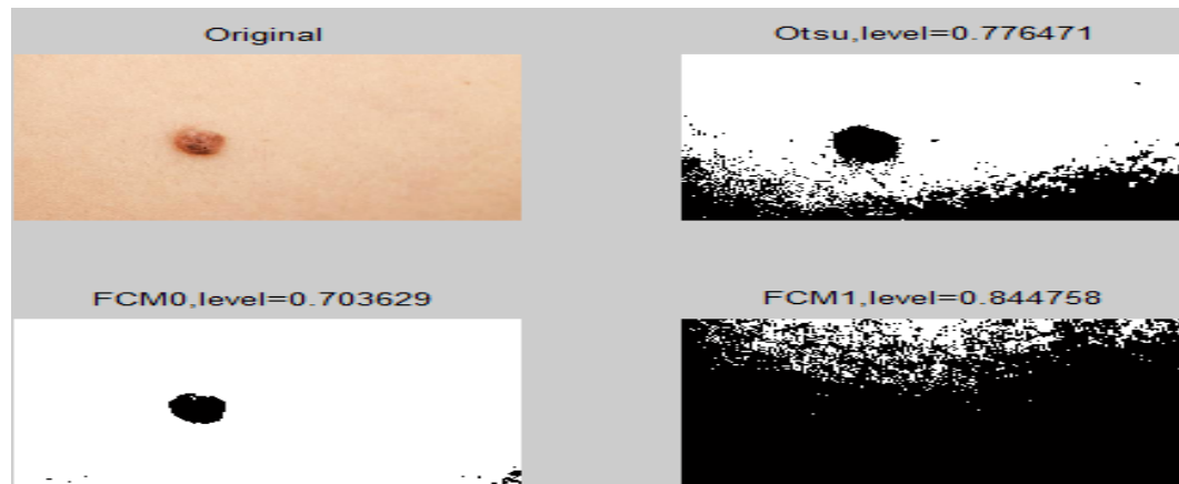
Figure 4: Segmentation of image 1 (a) Original image (b) Otsu approach (c) FCM(Fuzzy C-means) (d) FCM1
