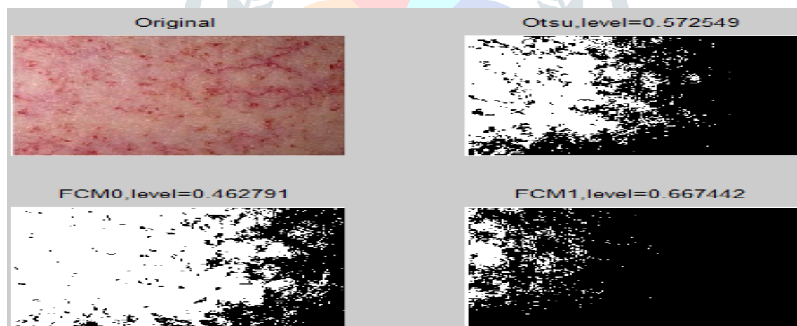
Figure 5: Segmentation of image 2 (a) Original image (b) Otsu approach (c) FCM (Fuzzy C-means) (d) FCM1
