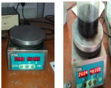
Figure 5 Mixing of epoxy resin and fly ash on magnetic stirrer
