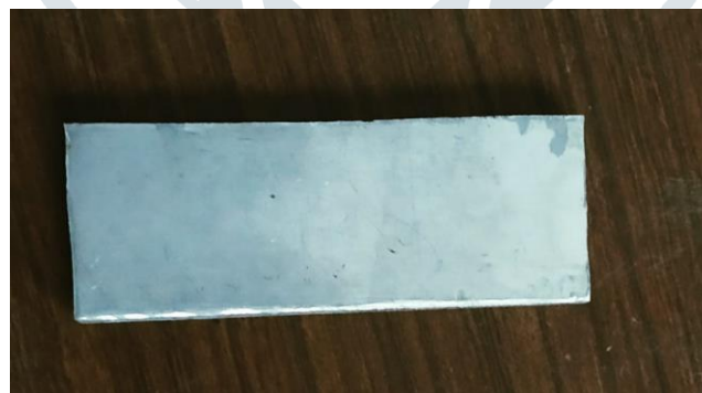
Fig:1.Sample work material(aluminium alloy 6082)
