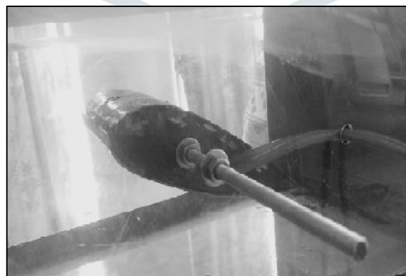
Fig .6: Boundary layer separation at 50^\circ angle of attack
