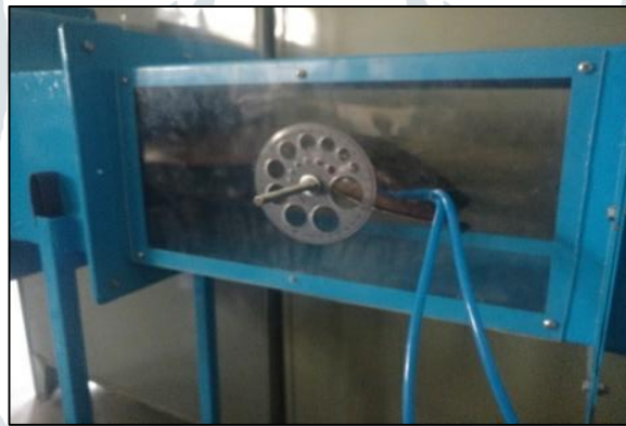
Fig.5: Experimental setup with wall mounted aerofoil
