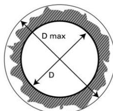
Figure 3 Pictorial view of delamination
