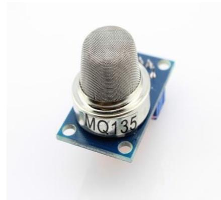
**Fig 4: Gas sensor(MQ135)**
