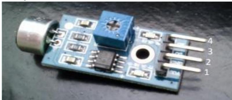
**Fig 5: Sound Sensor and its Pin-Out**
