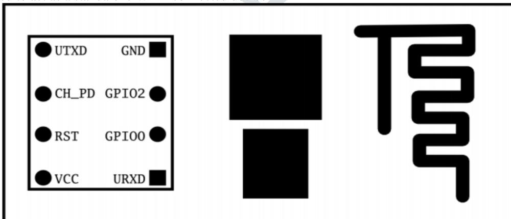
**Fig 6: Wi-Fi module and pin out (ESP8266)**
