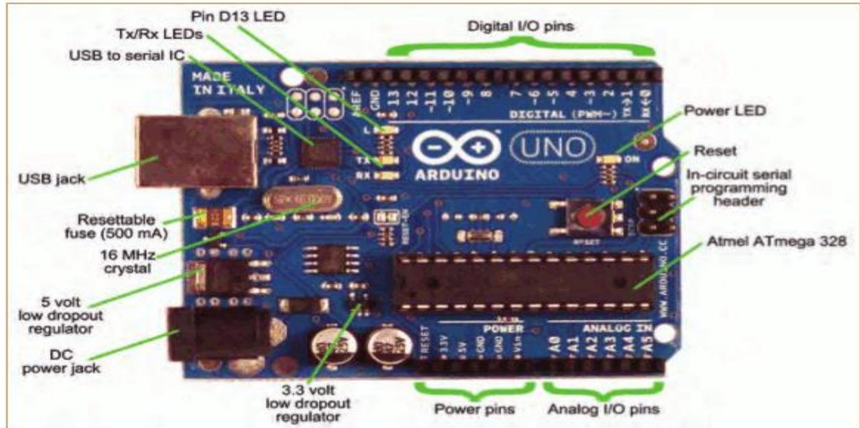
**Fig 3: Arduino Uno board**
