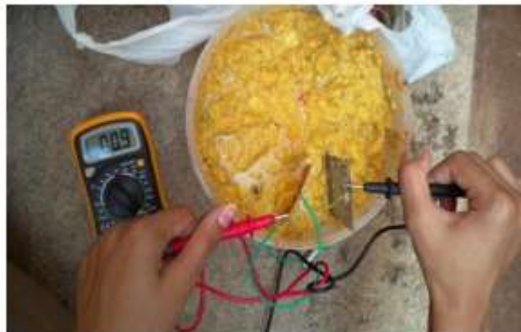
Fig2 Voltage reading for a single pair of Zn-Cu electrode
