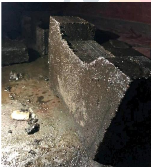
Fig: 4.4.4.Demoulding of Paver blocks from Mould
