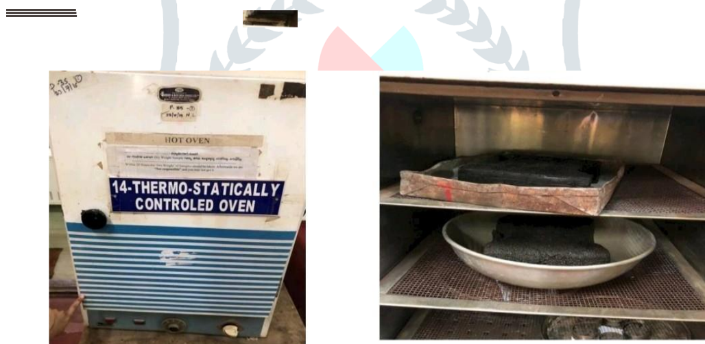
Fig: 4.5.2.Oven Test for Mould
