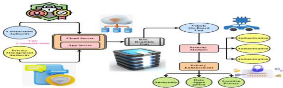
Figure.2: Framework for the proposed IDS for VANETs.
