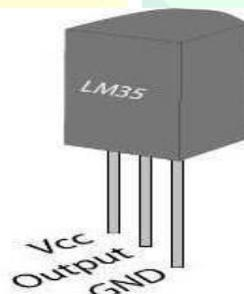
Fig 5. IC LM35 Temperature Sensor
