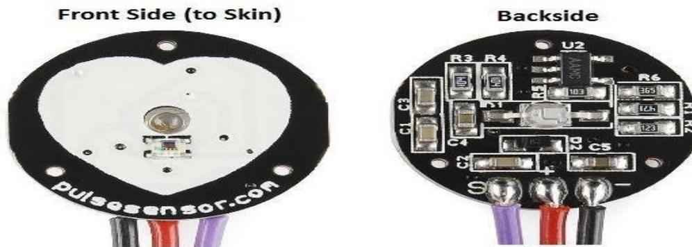
Fig 4. Pulse Sensor
