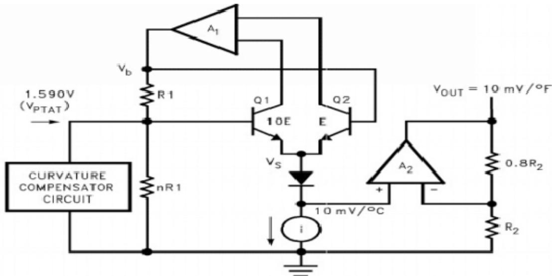
Fig 8. Internal circuit of IC LM35 Temperature Sensor
