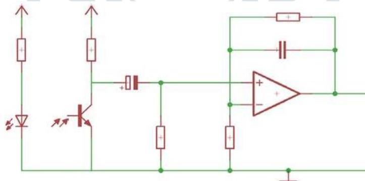
Fig 7. Internal circuit of Pulse Sensor
