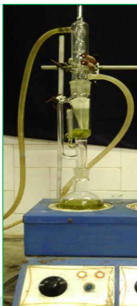
Fig-1 Sample preparation on the Soxhlet extraction method
