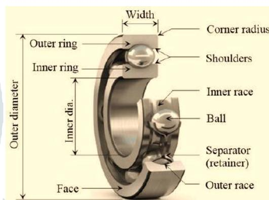
Camshaft Bearing Bigger End code: 6203
