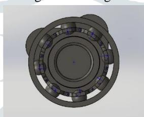
Fig 1.3 Camshaft bearing modified with protective shield
