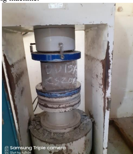
Fig.6 Concrete cubes (150mm*150mm*150mm) in Compression test machine (CTM)
