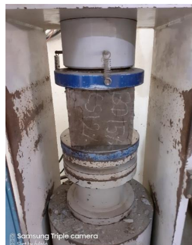
Fig.6 Concrete cubes (150mm*150mm*150mm) in Compression test machine (CTM)
