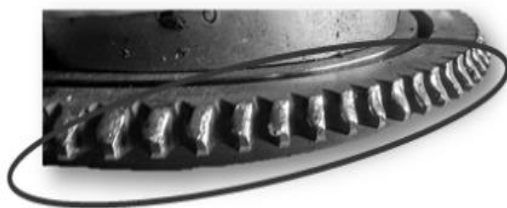
Fig 1.3 Before modifying Flywheel ring gear
