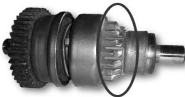
Fig 1.4 Pinion Gear without chamfer
