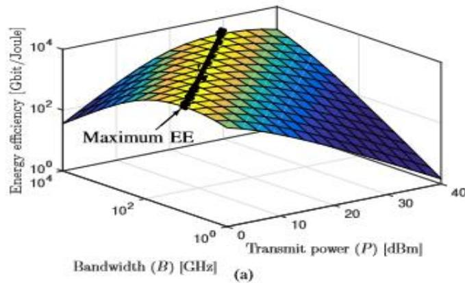
Fig: The EE in(a) vary with the transmit power and bandwidth.
