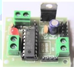
Microcontroller cannot supply the current required to run DC motor. So satisfy this requirement IC’s are used to drive the motor. The L293 and L293D are quadruple high current half –H drivers.
