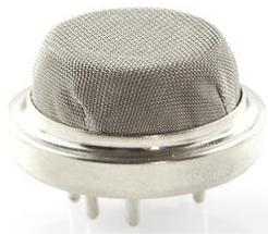
This is a simple-to-use liquefied petroleum gas (LPG) sensor, suitable for sensing LPG (composed of mostly propane and butane) concentrations in the air. This sensor has a high sensitivity and fast response time. The sensor's output is an analog resistance. The drive circuit is very simple; all you need to do is power the heater coil with 5V, add a load resistance, and connect the output to an ADC.
