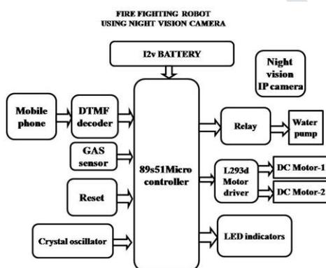
Here the working starts with the directions given by the user through the mobile. Here, the two mobiles are utilized. One is to send the DTMF signal and the other to receive these signals. The signals are nothing but the mixer of the double tone multiple frequency signals. A mobile phone lead is utilized at the receiver circuit to feed the signals from the mobile to the DTMF circuit. The DTMF(double tone multiple frequency) IC is capable of resolving the different-different signals
