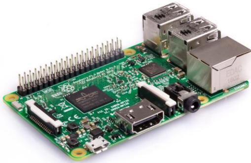
The Raspberry Pi 3 Model B is the latest single-board computer from the Raspberry Pi Foundation. In this version, they've upgraded to a 1.2 GHz 64-bit quad-core ARM processor and added 802.11n Wireless LAN, Bluetooth 4.1 and Bluetooth Low Energy.
