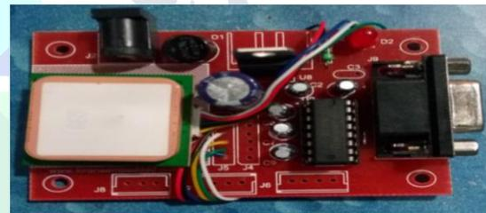
The GPS Receiver consists of two units, first is active antenna which receives RF signals and amplifies it. The antenna is active in the sense it takes power from the module and amplifies the signal for high sensitivity. The RF signal is filtered and processed to generate NMEA format serial data output.
