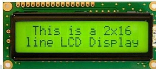
**Fig 3: LCD 2X16 MODULE**
