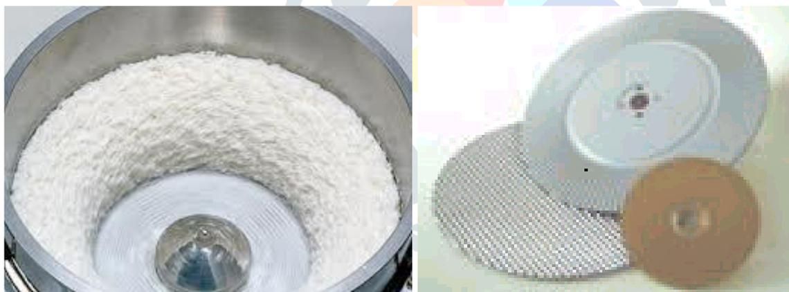
**Figure 2: Spheronization Process**
