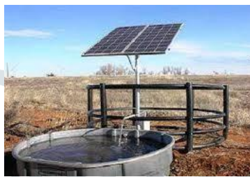
Figure 12 Application for Water pumping
