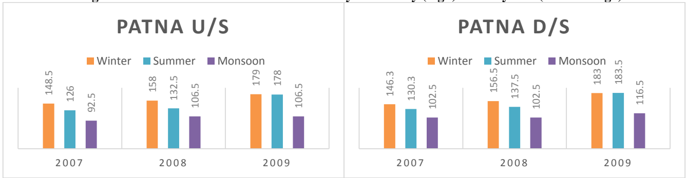
Fig 18. Trends of Seasonal Variation of Total Dissolved Solid (mg/l) at Study Site (River Ganga)
