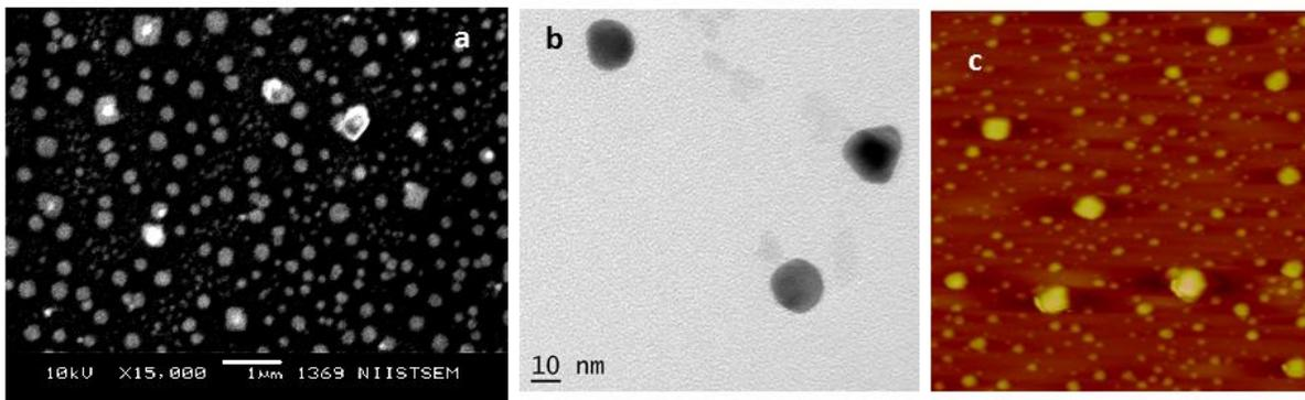
**Figure 5. SEM(a),TEM (b) and AFM (c) images of AgNPs.**
