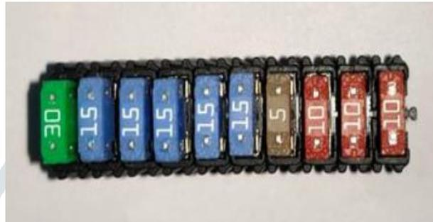
Figure 6: Non-Defective Fuse
