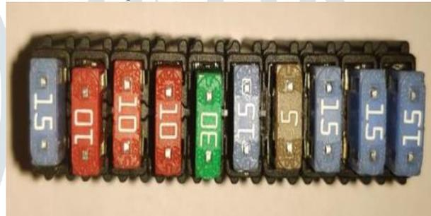
Figure 7: Defective Fuse (Incorrect Order)
