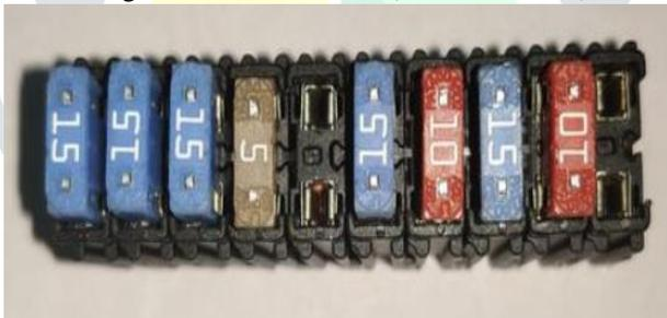
Figure 8: Defective Fuse (Missing fuse)
