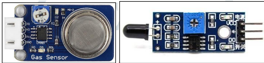
Fig 04. Smoke & fire sensors
