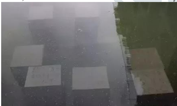
Fig 3 showing concrete cubes dipped in curing tank filled with water and chemical.
