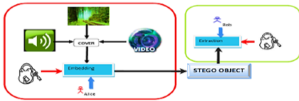
Figure 1: General schematic description of steganography with different types of covers
