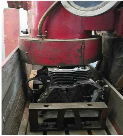
Fig.5 Surface grinding to increase CR
