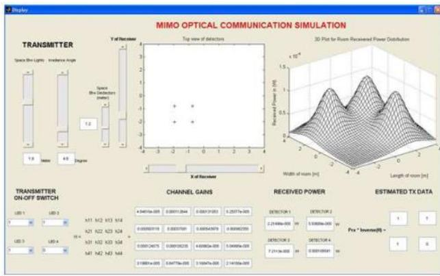
Figure 4: A gui model of MIMO and OFDM based Optical communication system
